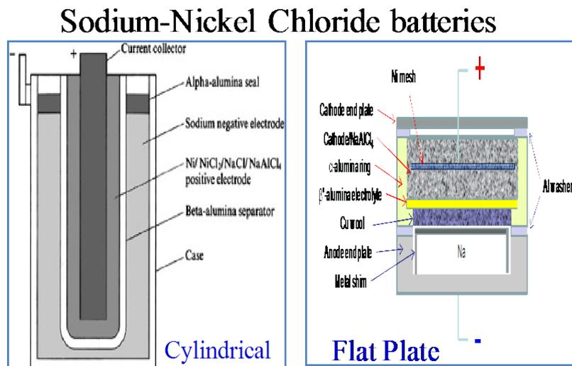
Figure 4-6. Schematic view of tubular and planar Na-MCl<sub>2</sub> batteries
