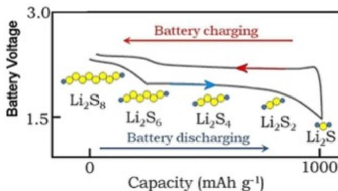
Figure 4-4. Reactions in a Li-S cell
