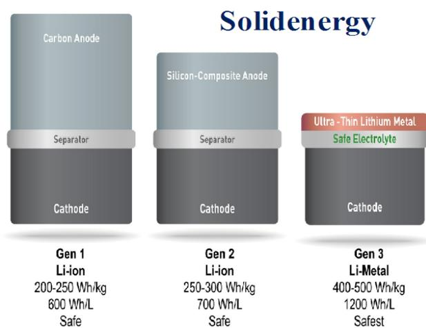
Figure 4-5. Projected performance of Li metal based technologies by Solidenergy
