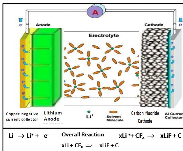
Figure 4-1. Chemistry of Li-CFx primary cell
