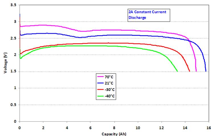
Figure 4-3. Performance of Li/CF<sub>x</sub>-MnO<sub>2</sub> D cell at different temperatures. The CF<sub>x</sub>-MnO<sub>2</sub> hybrid cathode allows operations over a wide range of  $-40^{\circ}\text{C}$  to  $70^{\circ}\text{C}$ .
