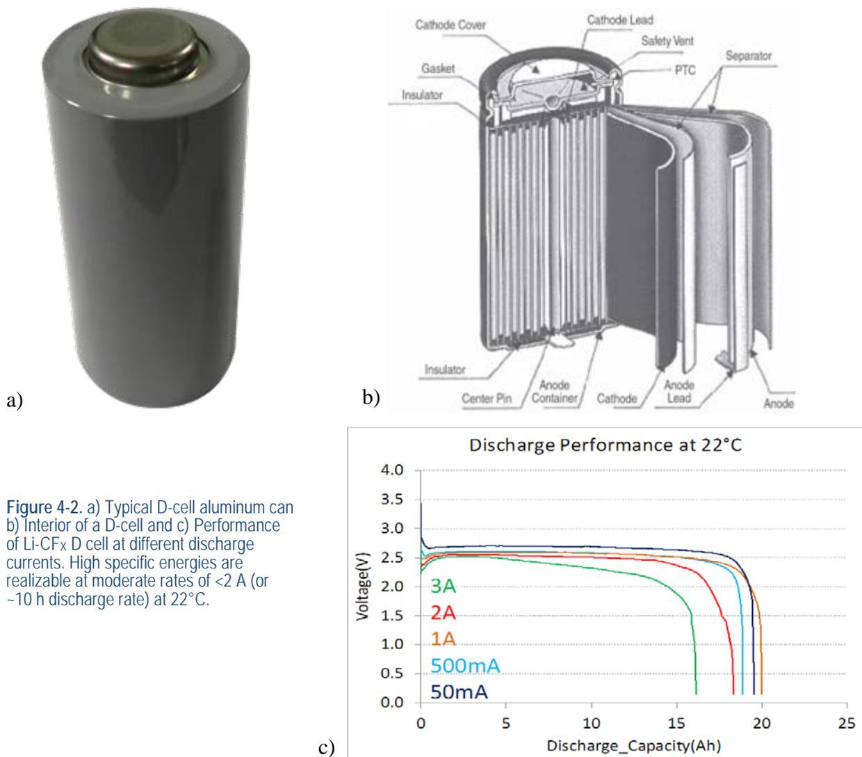
**Figure 4-2.** a) Typical D-cell aluminum can b) Interior of a D-cell and c) Performance of Li-CFx D cell at different discharge currents. High specific energies are realizable at moderate rates of  $<2$  A (or  $\sim 10$  h discharge rate) at  $22^{\circ}\text{C}$ .
