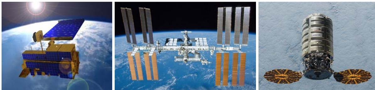
Figure 3-5. Flexible Fold-Out Arrays. *Left:* Illustration of Terra spacecraft with APSA based array.<sup>15</sup> *Middle:* International Space Station with eight flexible arrays and ~2500 m<sup>2</sup> total area.<sup>16</sup> *Right:* Cygnus resupply vehicle with UltraFlex array.<sup>17</sup>
