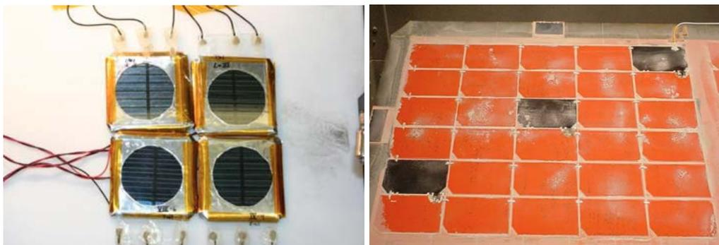
Figure 4-17. Martian Dust Mitigation Technology. At left is a technology utilizing electric fields for dust removal. At right is a technology using piezoelectric actuators and mechanical vibration.
