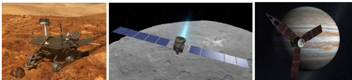
Figure 3-4. Deployable Rigid Arrays. From left to right: Mars Exploration Rover with 1.2 m<sup>2</sup> array, Dawn spacecraft (mission to Vesta and Ceres) with 36 m<sup>2</sup> array (illustration), Juno spacecraft (mission to Jupiter) with ~43 m<sup>2</sup> array (illustration).
