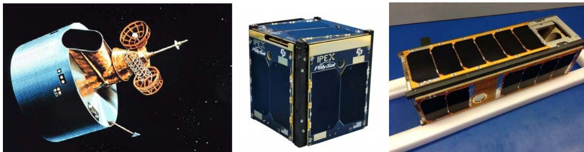
Figure 3-3. Body-mounted arrays. From left to right: GOES 7 (NASA/NOAA) spinning satellite (illustration), CP8 IPEX (Cal Poly Intelligent Payload Experiment, app. 10 cm × 10 cm × 10 cm), RACE (Radiometer Atmospheric CubeSat Experiment).
