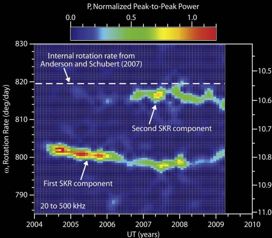
Saturn emits periodic radio signal, which are measured by the RPWS instrument onboard Cassini.
