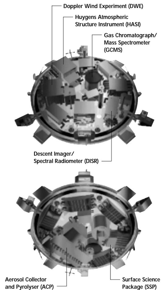
Detail of the probe's interior showing investigations on both sides.
