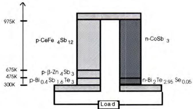
Figure 5.3.2-3. Schematic of First Generation Advanced Segmented unicouple at JPL
