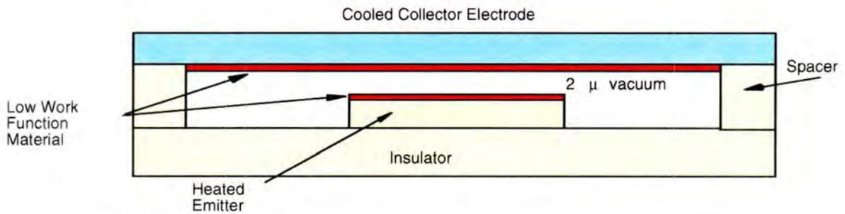
Figure 5.4.4-1. Sandia Microminiature Thermionic Converter (MTC)
