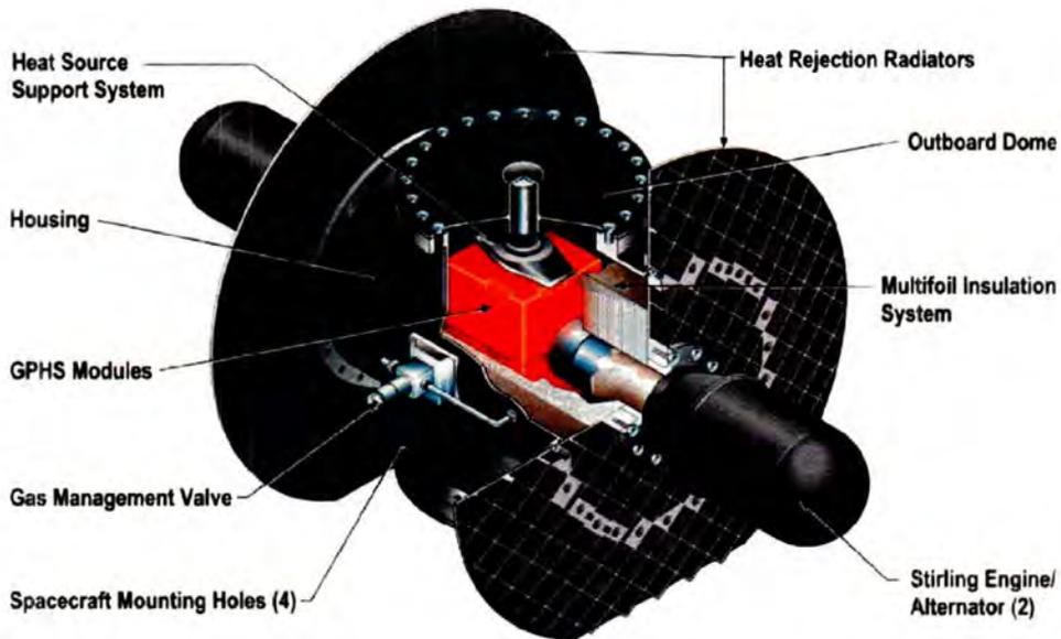
Figure 5.2-5. LMA 109 Watt BOM Stirling Generator Concept
