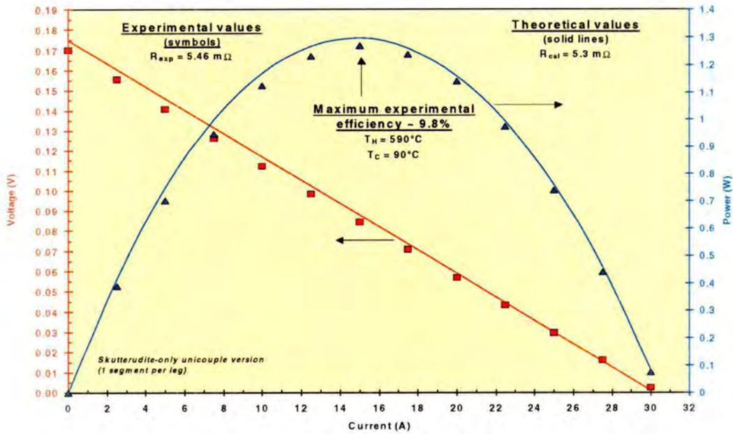
**Figure 5.3.2-5.** Recent data on a unicouple using a single skutterudite for the p-leg and  $\text{CoSb}_3$  for the n-leg
