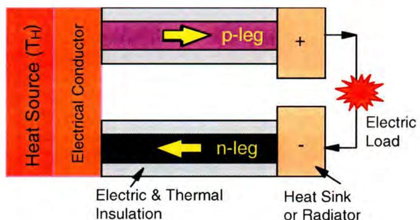
Figure 5.3.2-1. Schematic of a Thermoelectric Converter
