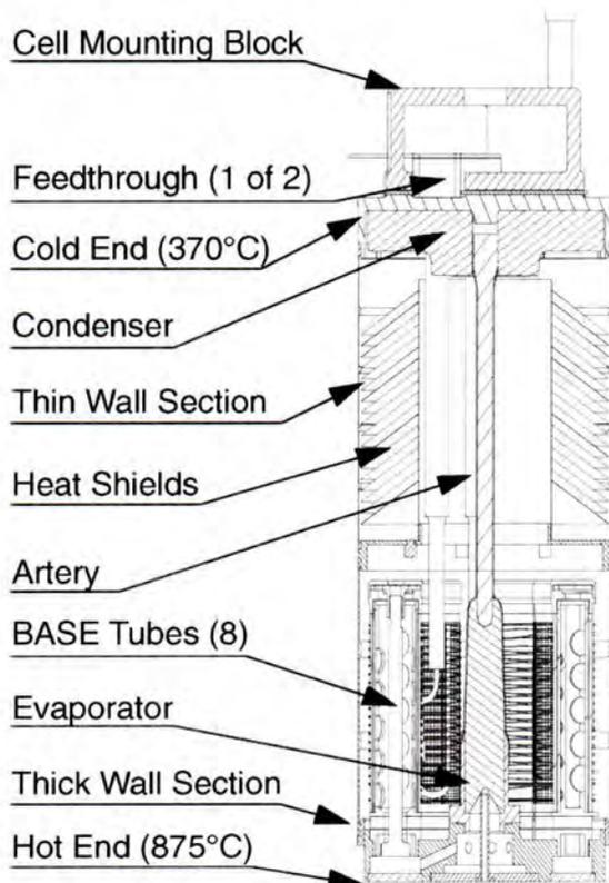
Figure 5.1-3. Current Cylindrical Converter Design
