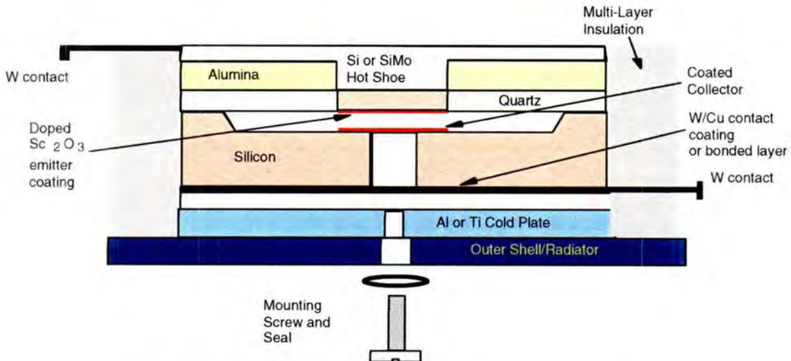
Figure 5.4.4-2. ARPS-MTC Configuration (not to scale)
