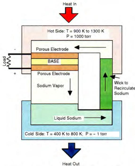
Figure 5.1-2. Schematic of AMTEC Cell
