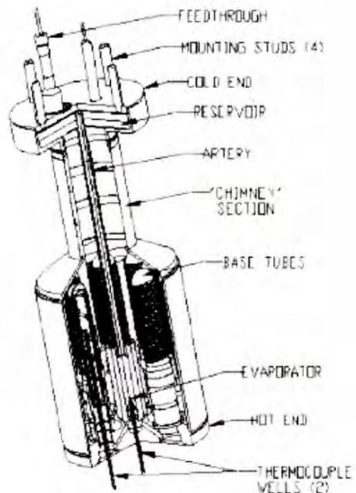
Figure 5.1-4. Chimney Converter Concept
