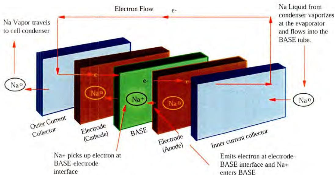
**Figure 5.1-1.** BASE, Electrodes, and Current Collectors Schematic
