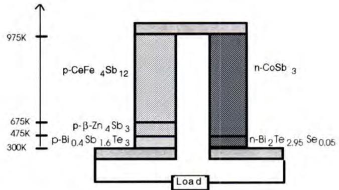
Figure 5.3.2-3. Schematic of First Generation Advanced Segmented unicouple at JPL
