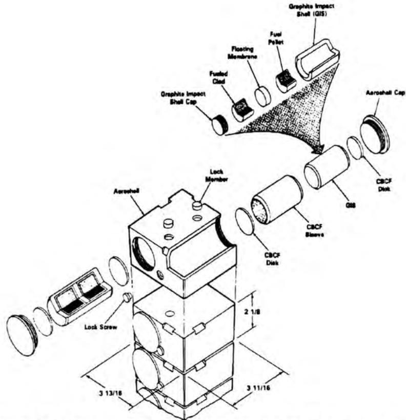
Figure E-1. Disassembled Impact Shell Holding Two Fuel Clads
