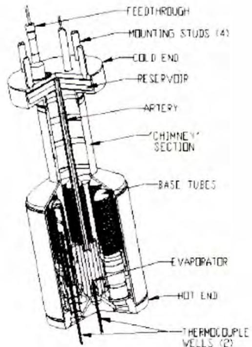
Figure 5.1-4. Chimney Converter Concept
