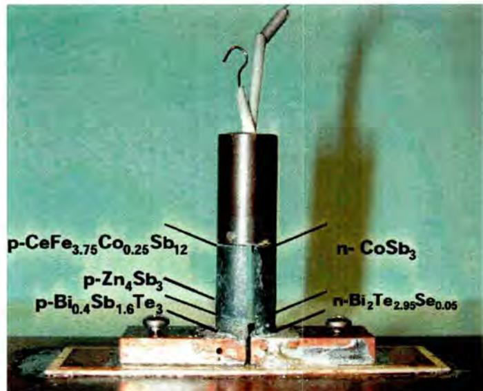
Figure 5.3.2-4. First Generation Advanced Segmented Unicouple Tested at JPL
