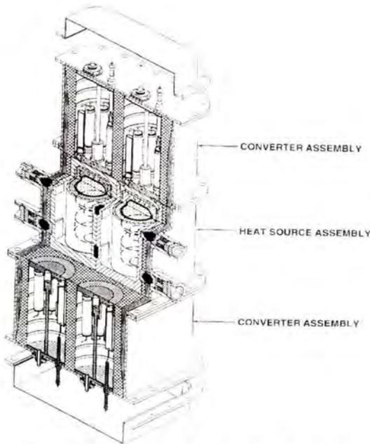
**Figure 5.1-6.** OSC 73.5 Watt BOM Conceptual Generator Design
