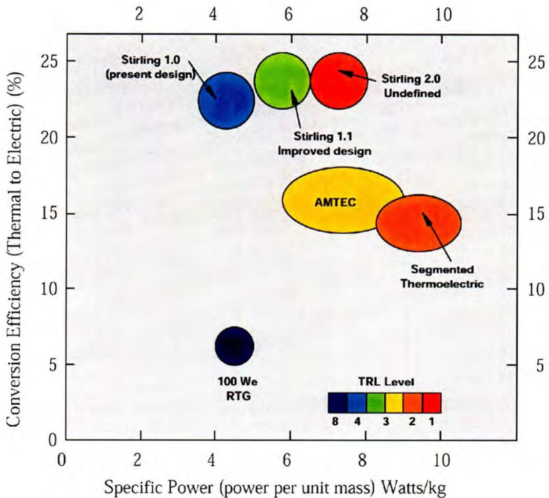
**Figure 6-1.** Comparison of Conversion Efficiency and Specific Power
