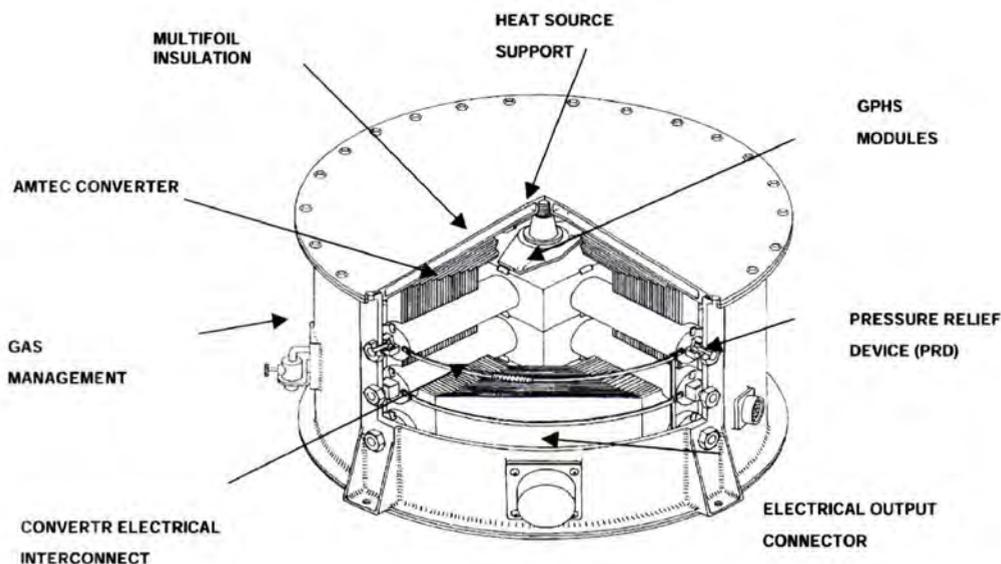
Figure 5.1-5. LMA 134 Watt BOM Generator Preliminary Design
