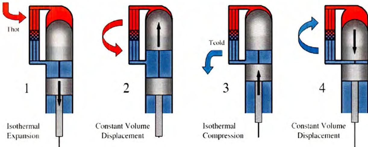
Figure 5.2-2. Stirling Cycle Thermodynamic Process
