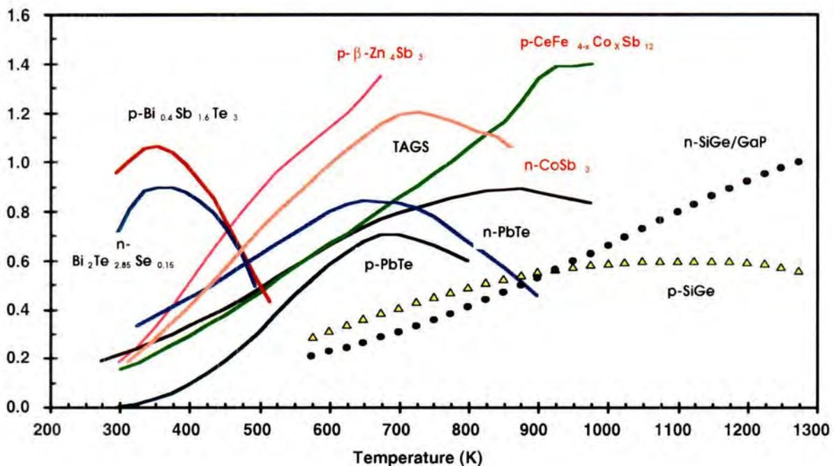
**Figure 5.3.2-2.** Thermoelectric figure-of-merit,  $ZT$ , as a function of temperature for state-of-the-art SiGe and  $\text{Bi}_2\text{Te}_3$ -based alloys and the new  $\text{Zn}_4\text{Sb}_3$ ,  $\text{CoSb}_3$  and  $\text{CeFe}_4\text{Sb}_{12}$  compounds.
