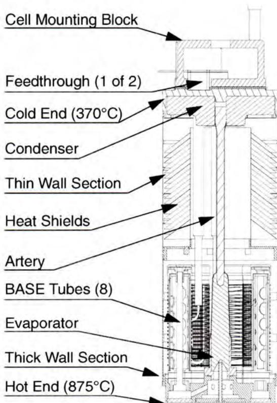
Figure 5.1-3. Current Cylindrical Converter Design
