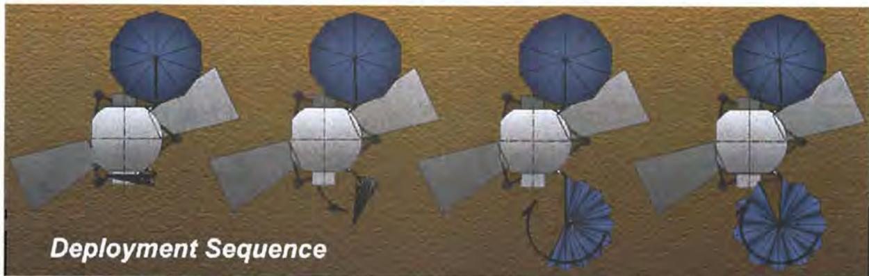
**Figure 5-3:** UltraFlex™ Solar Array Wing System for the Mars 01-Lander Spacecraft
