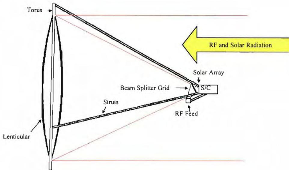
Figure 5-18. Inflatable Power Antenna Concept.
