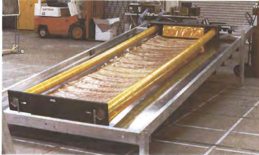
Figure 5-17. Deployment Test Setup Used In Thermal/Vacuum Chamber
