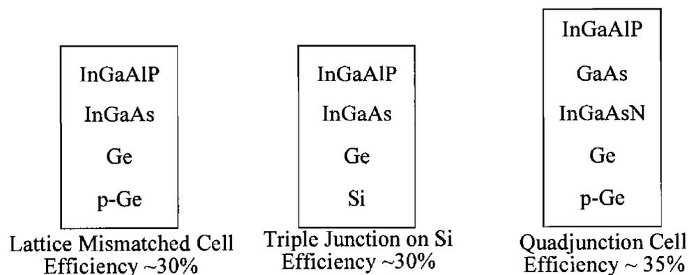
**Figure 5-1:** Conceptual Cell Designs. The lower most layer in each case is the substrate which does not contribute to power generation.
