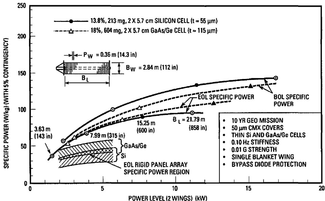
Figure 3-7: Projected Specific Power of the APSA Array with Various Cell Technologies
