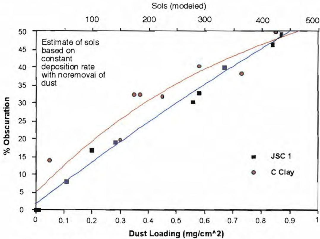
Figure 5-11: Measured extinction curve for two simulants to Mars dust. Vertical scale is the % power reduction due to dust loading.
