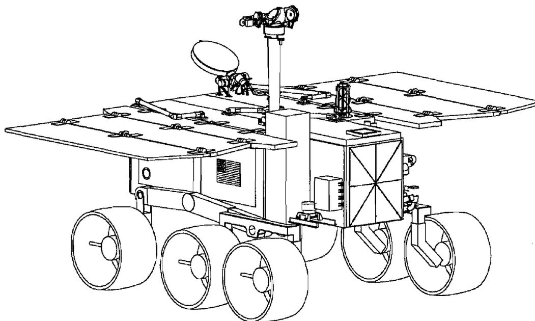
**Figure 4-2:** Conceptual Layout of Advanced Rover Showing Multiple Panels of PV Arrays Deployed
