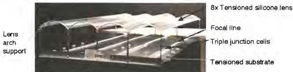
**Figure 5-10.** ABLE Stretched Lens Concentrator
