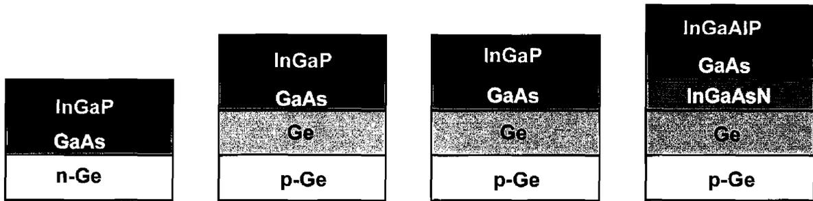
**Figure 3-3:** Schematic Representation of Double, Triple, and Quad Junction Solar Cells. The lowermost layer is the substrate and does not produce any electrical power.
