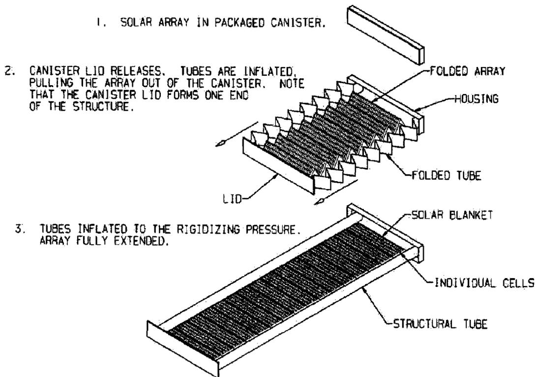
**Figure 5-16:** Inflatable Array Concept
