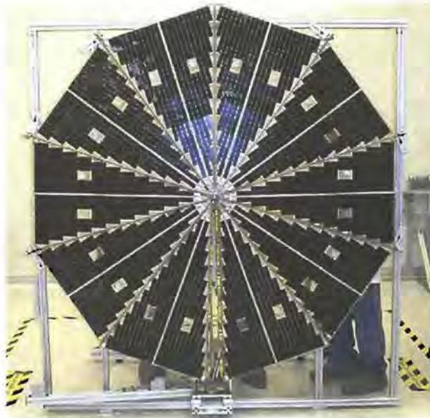
**Figure 3-6:** Flexible Round Panel Array With Circular Deployment
