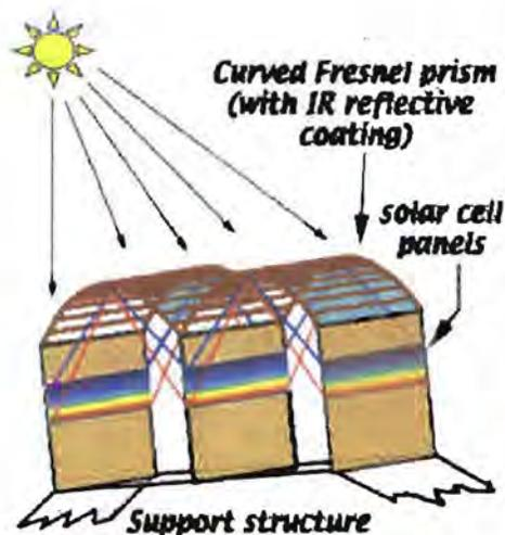
Figure 5-14. Multi-Bandgap High Efficiency Rainbow Converter
