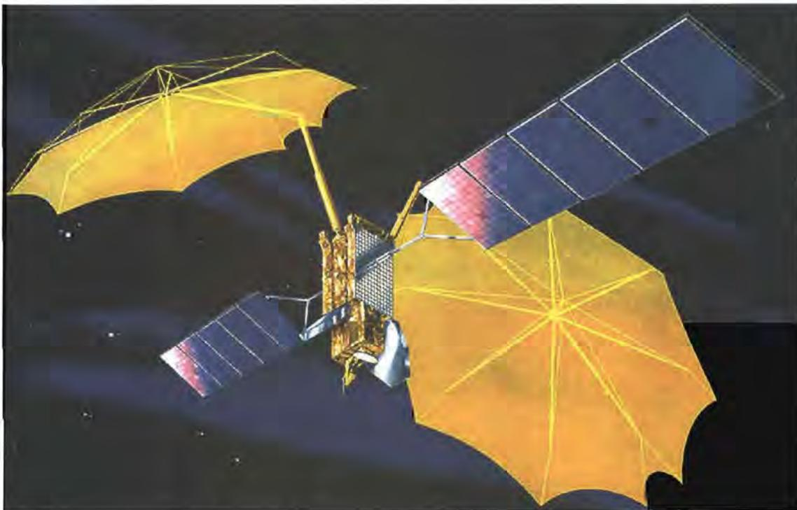
Figure 3-4 Rigid panel GaAs Solar Array
