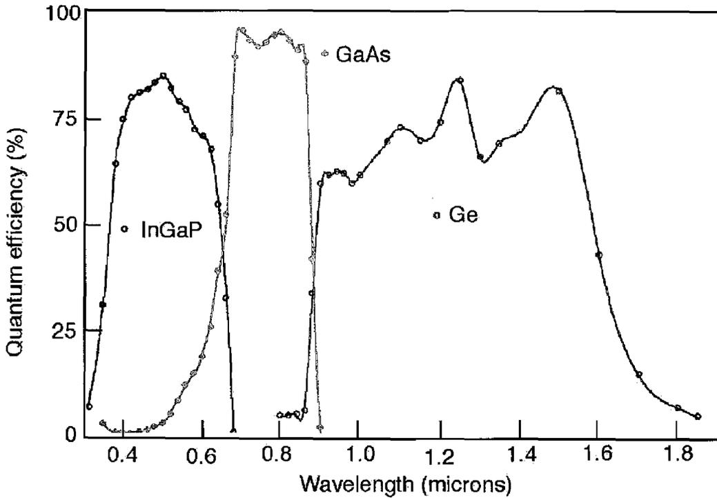
**Figure 3-2:** Quantum Efficiency vs. Wavelength for Each Layer of a Triple Junction Cell. The InGaP is the uppermost layer and it is used to convert the highest energy part of the spectrum.
