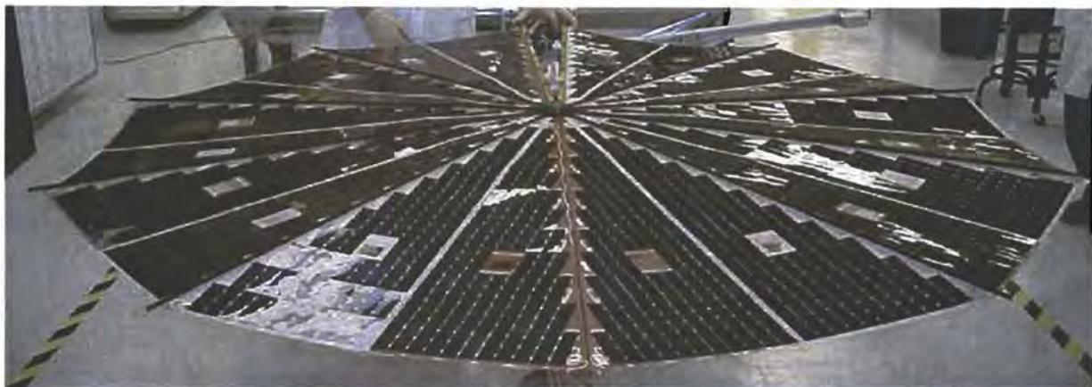
**Figure 5-4.** Ultraflex™ Array in Deployed Condition
