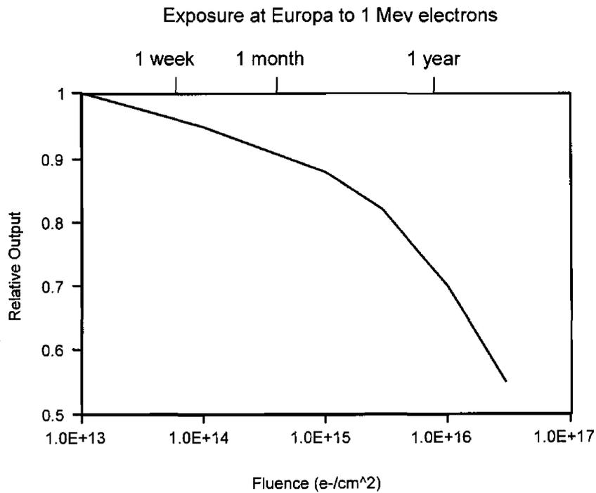
Figure 5-12. Relative output of 2-junction GaAs cell vs. fluence of 1 MeV electrons
