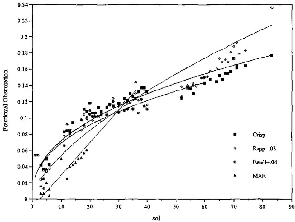
**Figure 4-3:** Pathfinder data on obscuration of a solar cell. The data marked Crisp, Rapp and Ewell are different interpretations of the same data on an exposed cell, whereas the data marked MAE is from the MAE experiment.
