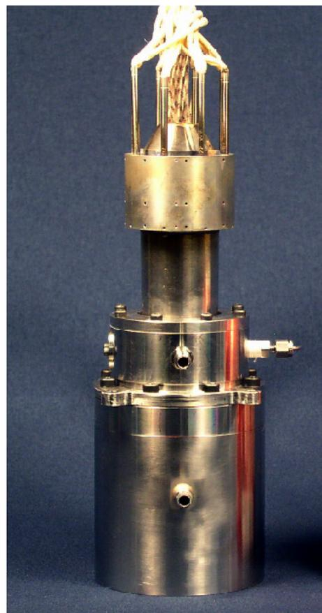
**Figure 3-6.** Laboratory Prototype of an Advanced 80 We SunPower Stirling Engine and Linear Alternator (Wood, 2005).
