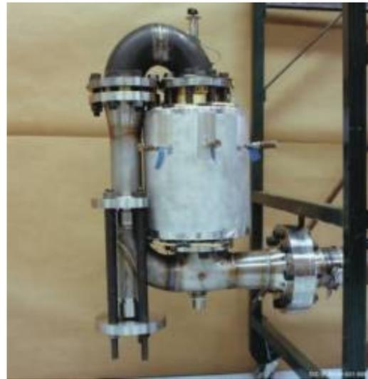
Figure 3-7. 1-kWe Engine and Resonator Developed by NGST and LANL (Petach, 2004b).
