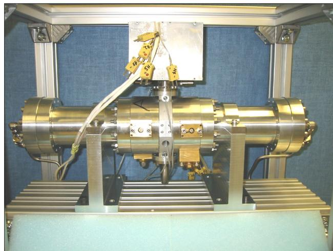
**Figure 2.5.2-5.** TASHE and Linear Alternator Operating at NGST (Tward, 2005)
