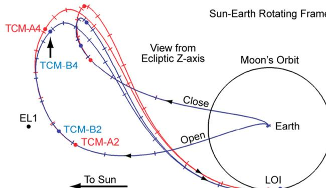
Figure 2.5-1. Trajectory design for the GRAIL mission, with multiple spacecraft elements.
