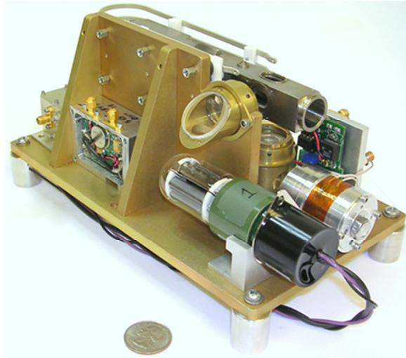
**Figure 3.1-1.** Laboratory brassboard version of DSAC in a low-mass and low-volume package; accurate to 1 ns in 10 days.
