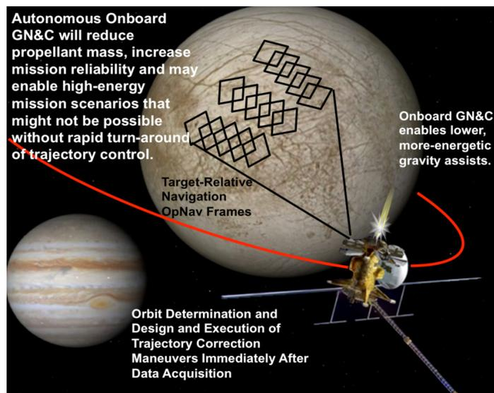
Figure 3.2-1. Autonomous onboard navigation for a Europa orbiter.
