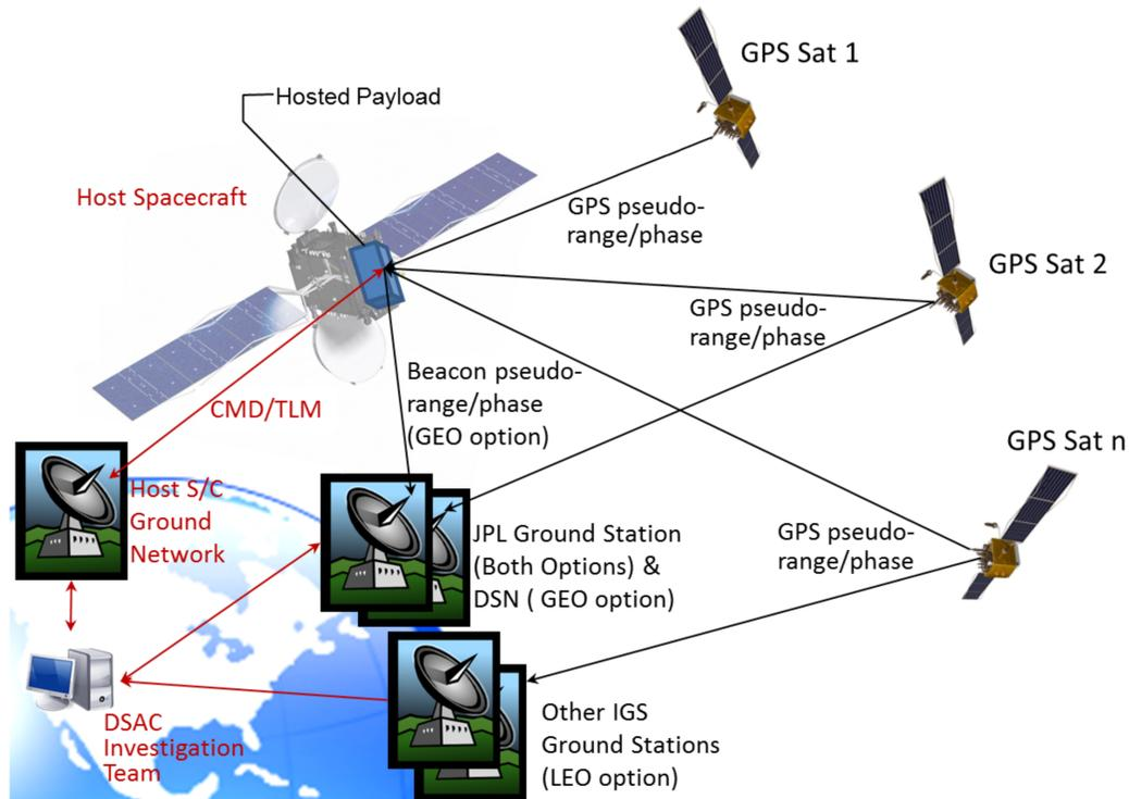
Figure 3.1-2. DSAC's Earth orbiting mission architecture.
