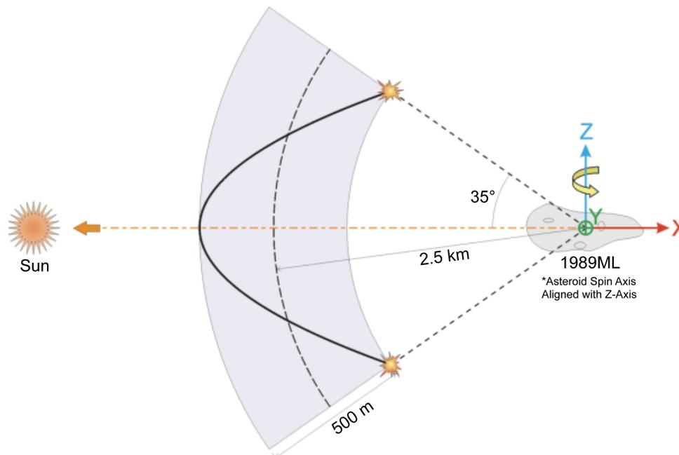
Figure 2.3-1. Close-proximity trajectory design for small-body missions.
