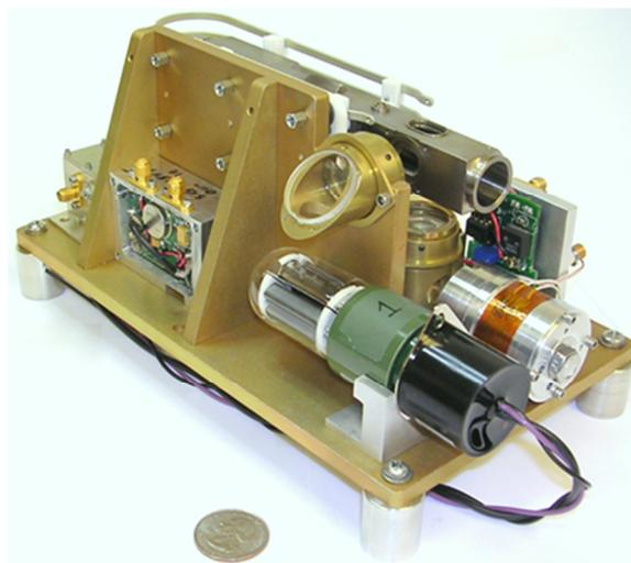
Figure 3.1-1. Laboratory brassboard version of DSAC in a low-mass and low-volume package; accurate to 1 ns in 10 days.
