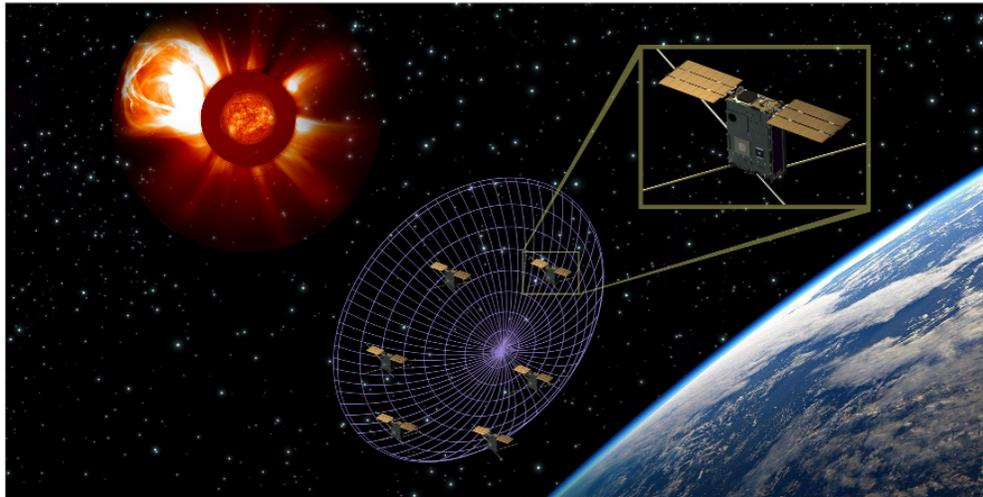
NASA's Sun Radio Interferometer Space Experiment (SunRISE) mission will send a fleet of six SmallSats into orbit around Earth to work together as one radio telescope to investigate radio waves coming from the Sun. By doing this, SunRISE will help scientists better understand space weather events.
