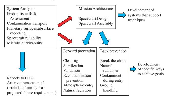
Figure 3.1-1. Framework for Analysis of Planetary Protection Technology Needs
