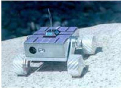
The MUSES-CN nanorover will be the smallest rover ever to fly on a space mission. (MUSES stands for the Mu Space Engineering Spacecraft--which is being built by the Japanese Institute of Space and Astronautical Science--C means it is the third in a series, and N stands for NASA's part in it, which is to build the nanorover.)
