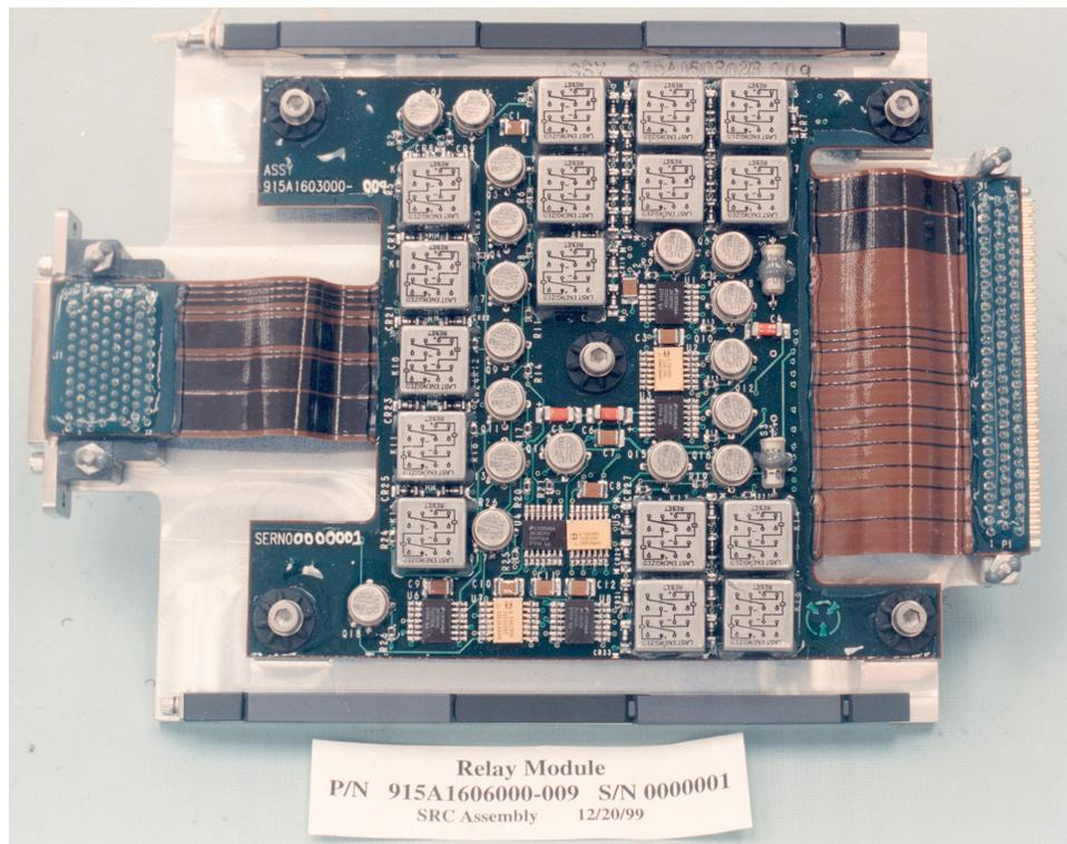
Figures 4.1 and 4.2 show an assembly drawing and close out photograph of a flight relay card with G-switch sensors, respectively.
