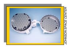
Solar Collector Wafers made of mostly silicon will be exposed to solar wind for two years.
