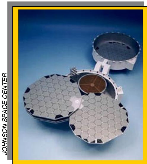
Genesis mission collector arrays and concentrator.
