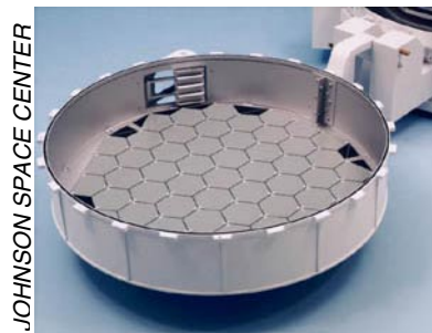
Genesis mission solar wind collector (2001).
