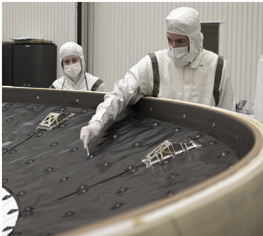
In a clean room at NASA's Kennedy Space Center, Mars Science Laboratory personnel sample the inboard side of the spacecraft's heat shield to confirm its cleanliness before final assembly for launch.
